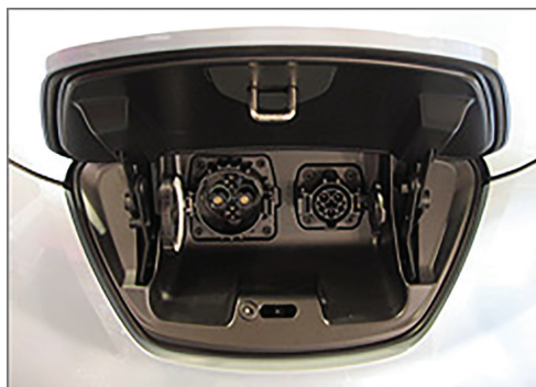
Figure 1. Photo shows a standard J1772 inlet on the right for use with Level 1 and Level 2 chargers; and a CHAdeMO inlet on the left. Photo from U.S. Dept. of Energy Energy Efficiency and Renewable Energy Website: ( http://www.afdc.energy.gov/fuels/electricity_infrastructure.html ).
